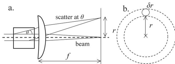
**Figure 1.** Optical principles of near-forward scattering measurements in the Fourier plane of a collecting lens.
