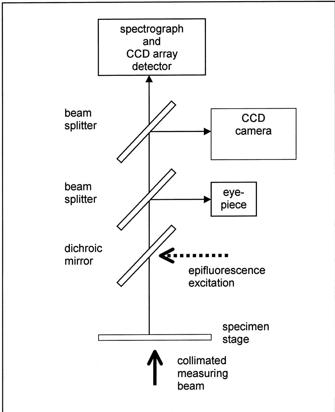
**Fig. 1.** Schematic optical arrangement of the modified microscope. The dichroic mirror was removed from the light path during absorbance measurements.
