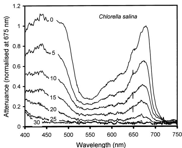
**Fig. 2.** Time course of photobleaching of a single diatom cell illustrated by consecutive measurements made at 5 s intervals. The graph displays the attenuation relative to a clear field of view, normalized at the red chlorophyll absorption peak of 675 nm for the initial measurement.
