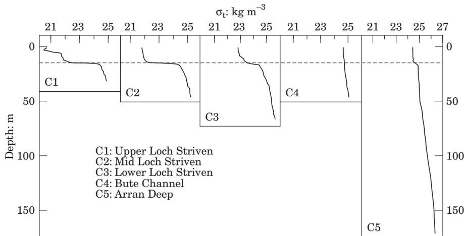
FIGURE 4. Density profiles for stations C1 (head of Loch Striven) to C5 (Arran Deep). The dotted line at around 15 m indicates the major pycnocline.
