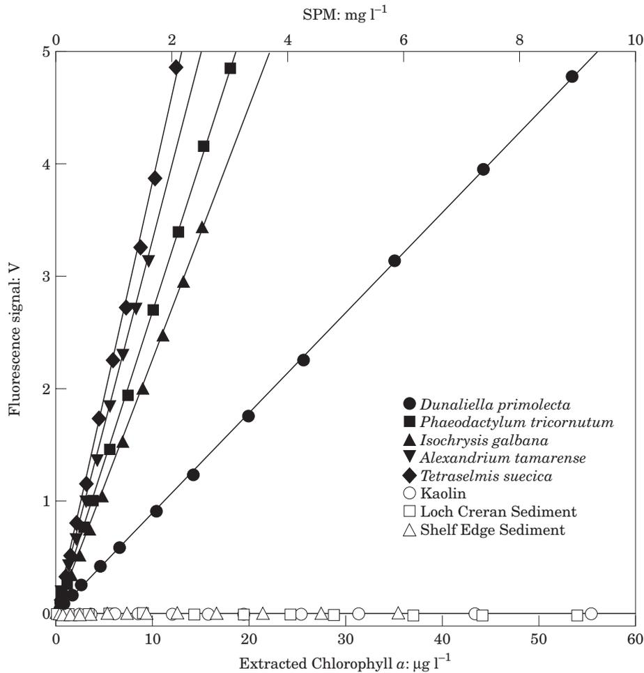
FIGURE 2. Response of the Seatech fluorometer to varying concentrations (expressed in terms of extractable chlorophyll) of five species of cultured phytoplankton. The negligible signals produced by scattering from inorganic particles are shown on a second x-axis.
